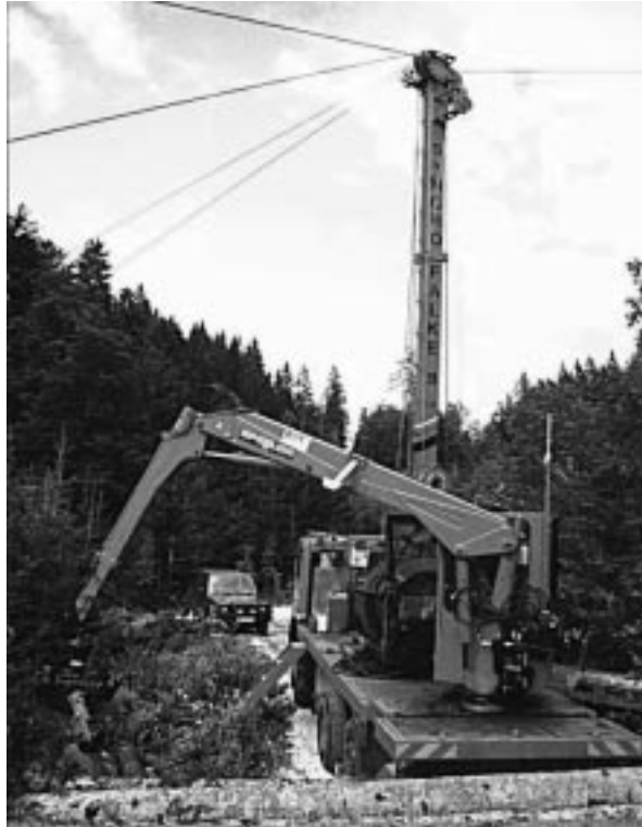
Figure 5: Syncrofalke automated yarder
